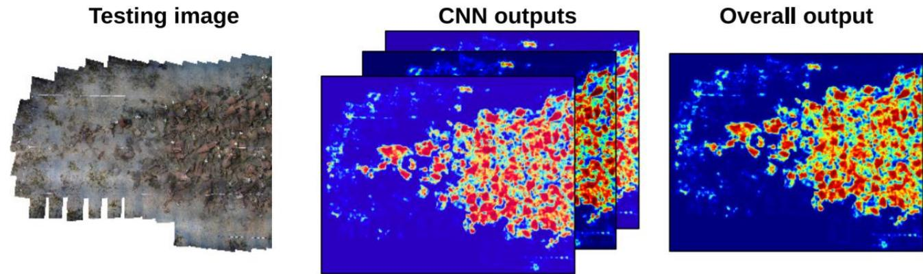
Each CNN apply the sliding window over the entire testing image
